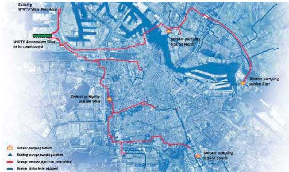
**Figure 1.1** Locations of the previous WWTPs Amsterdam East and South and the new WWTP Amsterdam West, with connecting pressure mains and booster pumping stations.
